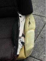
Once you have clear access then cut out the old foam along the line indicated below. Cutting from both sides as necessary in order to keep a nice clean cut to the line.
